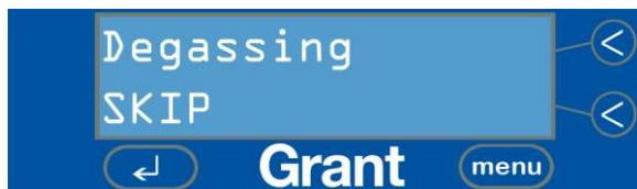
The degassing process is to remove all bubbles from the water as these impede the cleaning performance. Once all of the bubbles have come to the surface, complete the degassing cycle by pressing the  $\leftarrow$  key.
