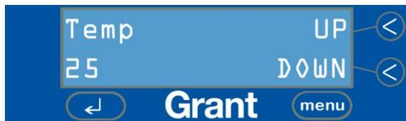
Use the UP and DOWN keys to accurately set the desired temperature of the cleaning liquid between ambient and 70°C.
