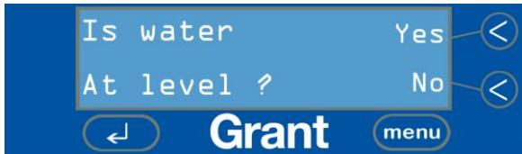
When the level sensor is disabled the liquid set temperature is automatically reduced to 5°C. The set temperature may be increased by entering the MENU system (see page 9).
