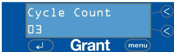
The cycle count shows all cycles which the bath has begun and includes those cycles which are not completed; i.e. those cycles aborted by the operator or because the liquid level was low.
