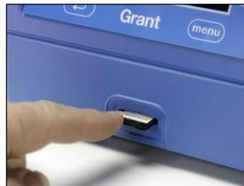
By recording to an MC card and transferring to a PC, a permanent electronic record of the cleaning cycle parameters can be saved.
