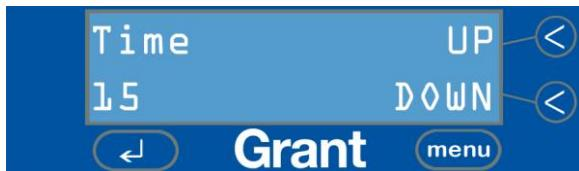
When the desired cycle time has been selected, use the MENU key to move to the next screen. This time setting will be saved until changed again in the Operator menu.
