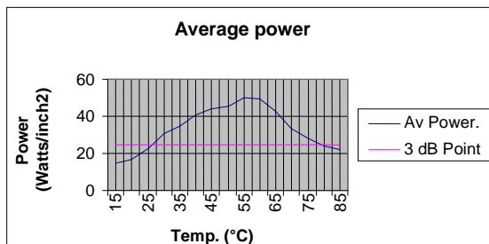
Ultrasonic activity itself will heat up the liquid at a rate of approximately 10-15°C per hour if in continuous use. In order to heat the liquid in the tank at a faster rate, it is recommended to run the ultrasonics as well as turn on the heating.
