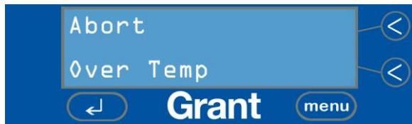
If the internal heater exceeds its allowed maximum, the following screen will be displayed.
